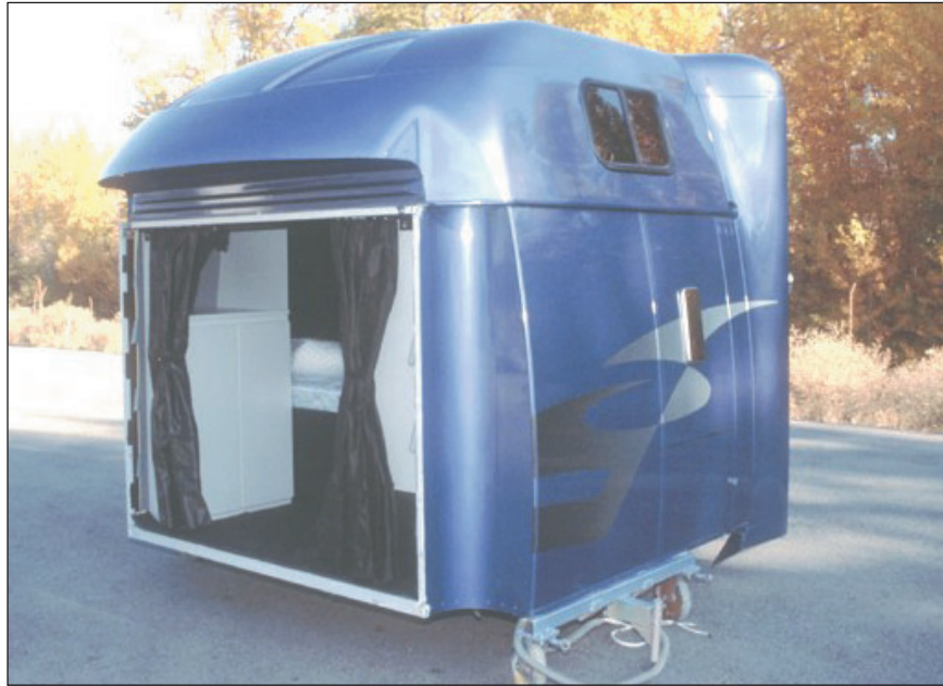
LIGHTWEIGHT: CCV continues building Western Star sleepers at its Kelowna, B.C. plant. They are about 850 lbs lighter than some other sleepers.
